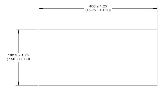
Figure 4: Panel Cutout Dimensions For Panel Mount Option
