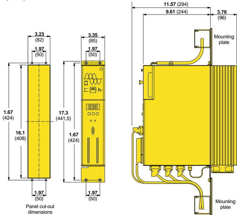
All backplate and bracket fixings accept M6 screws.
