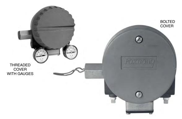
The E69F Field-Mounted Current-to-Pneumatic Signal Converter accepts a standard direct current input signal and converts it to a proportional pneumatic output signal for use with other pneumatic instruments or control valves. As symbolized by the "CE" Logo marking on the product, this product conforms to the applicable European Union Directives.
