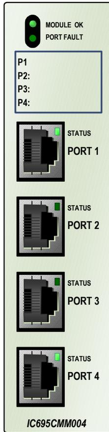
The Module OK LED indicates the status of the module. Solid green indicates that the module has been configured. The Module OK LED is off, if the module is not receiving power from the R3i backplane, or if a serious module fault exists.
