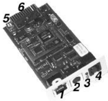
Figure 1.5.2 Internal SNMP Adapter
