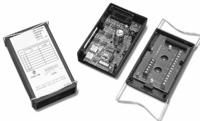
GALAXY SC provides peripheral monitoring and control through a local area network of small modules, which can be added as needed and mounted in the frame with the or placed near the measurement or control point.
