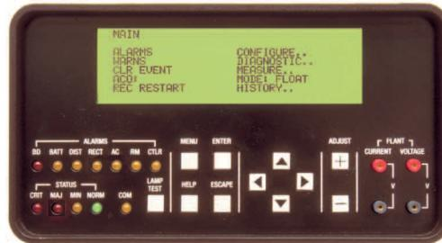
The front panel provides a backlit LCD display with an easy-to-use push-button, menu-driven interface. The panel can be used to program basic functions and access real-time data, history, statistics, and measured values.
