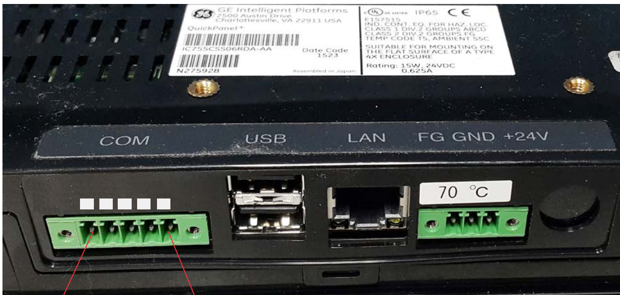
IC755CxS06RDx Serial Port COM1 Pin-out
