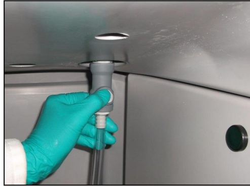
Figure 7: Removal of drain tubing
