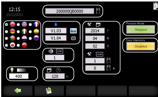
Operator access level screen
