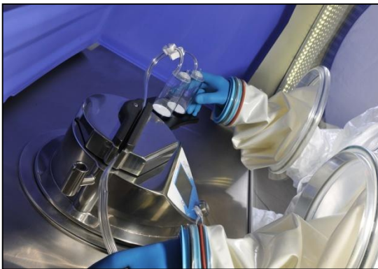
Figure 4: Sterility test unit in use (Equinox shown)
