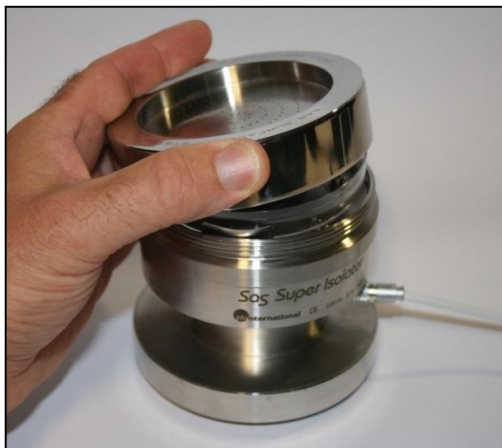
Figure 28: Removal of aspirating head
