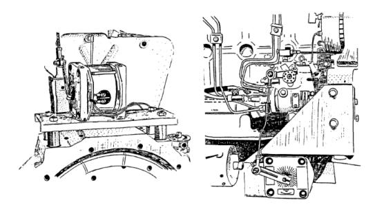
Figure 1. Typical EPG Actuator Installations
