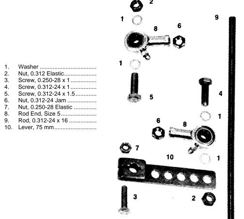
Figure 2. Parts Included with Linkage Kit 8924-370
