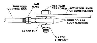
Figure 5. Rod End/Lever Assembly
