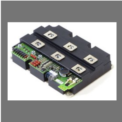
Drives IGBTs From 1200V To 3600V / 800 A To 3600 A
