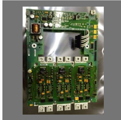
Siemens A5E01283291 IGBT With Driver Board 6sl3120-lte-28-5aa3 Power Pack
