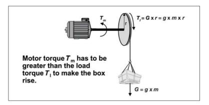
The load, friction and inertia resist rotation
