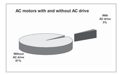
At the moment there are still plenty of motors sold without variable speed AC drives. This pie chart shows how many motors below 2.2 kW are sold with frequency converters, and how many without. Only 3% of motors in this power range are sold each year with a frequency converter; 97% are sold without an AC drive.
