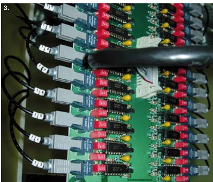
1. Magnetic field sensor | 2. Voltage sensor and RC circuit details | 3. Diagnostics main board for voltage sensors
